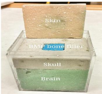
Fig. 3. Fabricated phantom.
